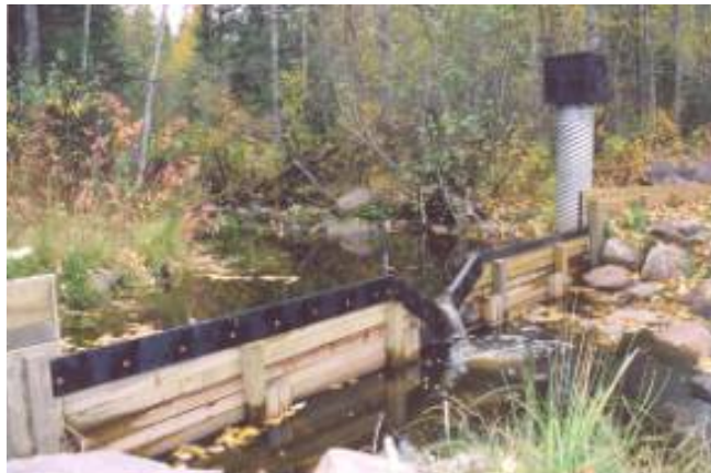
Figure. V-notch weir and stilling well, installed as part of the infrastructure for evaluating stream discharge and water quality for selected watersheds within the Dog River-Matawin Forest Management Unit.
